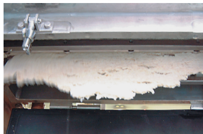
◆最終圧搾部でのおからの分離(二次搾り) Separation of TOFU refuse in the final pressing part (secondary pressing)
