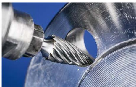
● A high-quality carbide cutter featuring a unique blade shape specially designed for efficient cutting of stainless steel. It is also suitable for grinding work materials that easily clog, such as aluminum.
